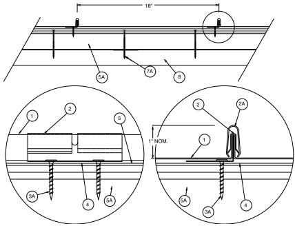
1. **Metal Roof Deck Panels\* -** No. 24 MSG min coated steel panels. 18 in wide, 1-1/2 in. high at ribs. Panels continuous over three or more clips with no endlaps. A bead of sealant may be used at panel side joints.
